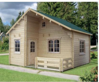
The design features of the Manhattan log cabin holiday chalet are akin to the log cabin designs that frequent the French Alps, and the close-grained 70mm logs used for the walls would be adequate for Alpine weather conditions too. Their dense grain maximises their insulation properties, and creates a durable, robust build. 570
